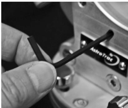
Ensure the latitude fine adjust knob is wound roughly half way into the latitude fine adjust bar so there is sufficient travel
